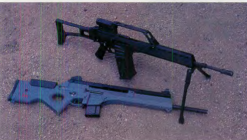
The semi-automatic SL8-1 (below) is seen with its selective fire G36 counterpart.
